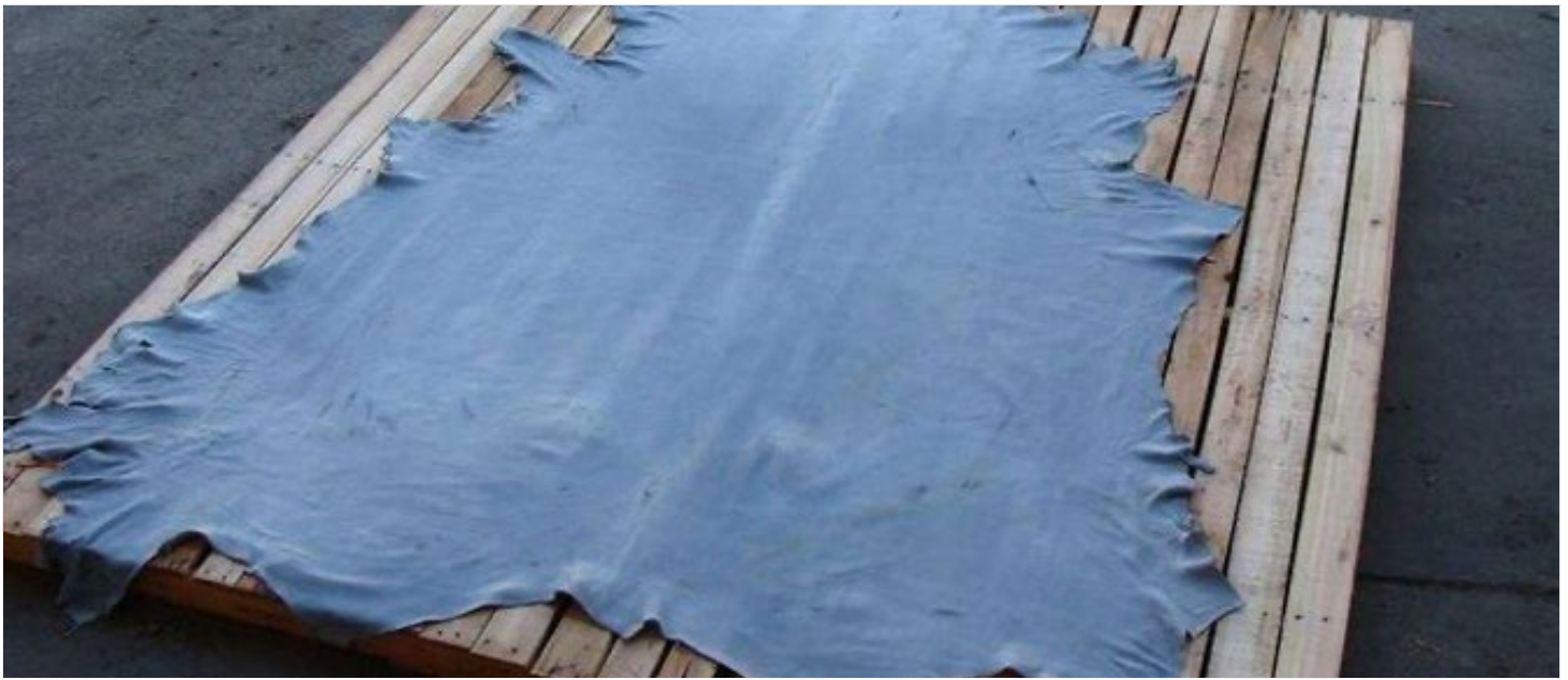
Figure 12. Wet blue animal hide preservation method. Credit: Leather Hide Council of America
